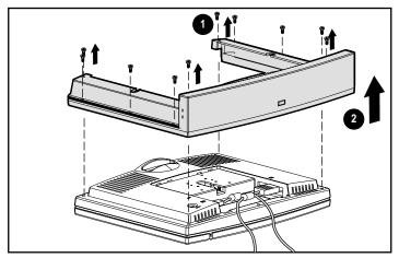
Figure 2-17. Removing the plastic frame
